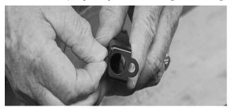
compound on the screw threads. Start the hexhead screw into the threaded sight shaft, ensuring the screw goes in straight. Tighten until it's snug, but don't overtighten the tiny screw.
