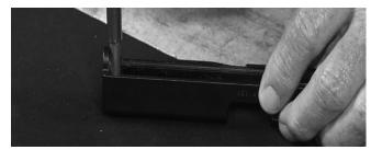
3) Check the alignment to make sure the front blade sits flush and square on the slide.
