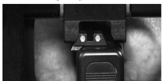
6) Center the sight on the frame, and check its alignment with the new front-sight post and tritium capsule. When you go to the range, take the MGW tool with you to make small horizontal sight changes.
