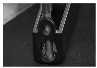
2) Insert the blade of the Tru-Dot front sight into the oval cutout at the front of the slide. The Tru-Dot blade should fit snugly. Place the hexhead screw into the Ed Brown tool, and put a tiny bit of medium strength threadlocking
